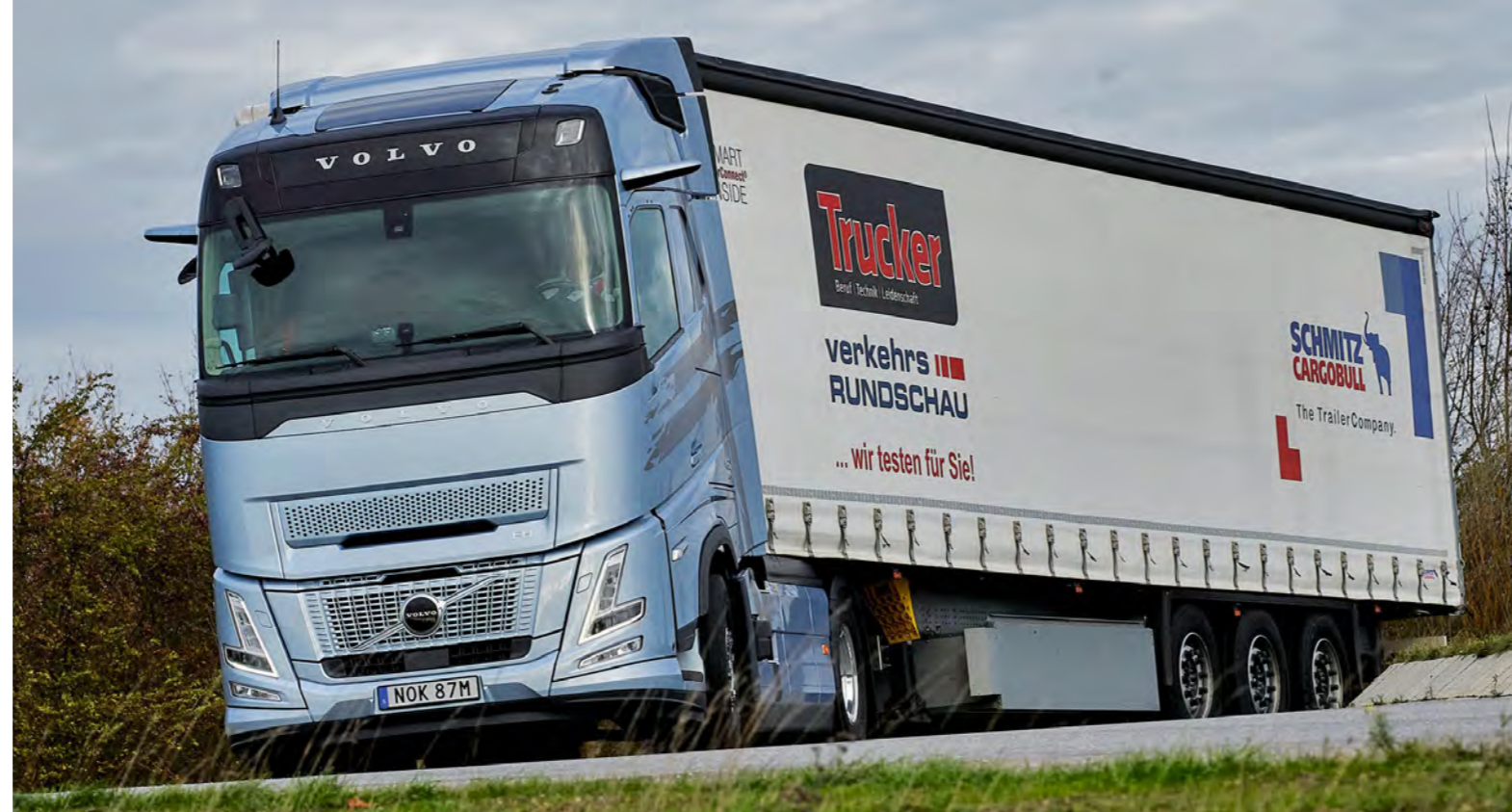
The Aero nose adds 60 kilograms of weight compared to the standard FH
