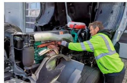
Compound Turbo turbine on right side
